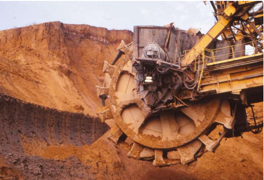
General view of the Chabařovice mine after the end of the mining activities, Retractable wheel excavator KU 300 mining a coal seam, author: Ing. Stanislav Štýs
